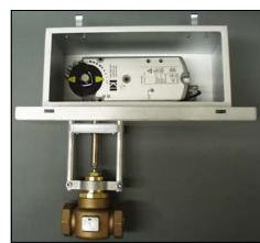
Construction: The enclosure is constructed of sturdy marine grade aluminum .080-inch (2 millimeters) thick. Any seams are continuously welded and ground smooth, and a corrosion resistant coating is applied to the entire enclosure for an extra degree of protection. The cover is secured with two quick release latches which allow easy access for maintenance.
