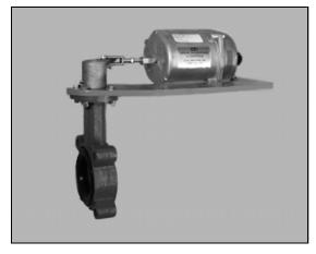
The Pneumatic Piston Type Spring Return Actuators provide actuation on butterfly valves in sizes up to 10 inches. These actuators are sized and installed for 70° disc rotation and require 20 to 30 PSIG (140 to 210 kPa) maximum input air pressure at the diaphragm to deliver the rated torque output.
