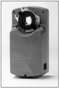
The EN "E" Series is a direct-mount line of actuators that operates on 24 VAC or VDC power and is available for use with resistive controllers. These bidirectional actuators do not require a damper linkage and are easily installed on a round shaft up to a 3/4" (20 mm) diameter or a square shaft up to 5/8" (16 mm). They can also be mounted to valves (ball, globe, and butterfly) using one of the many valve linkage kits available through Dodge Engineering & Controls.
