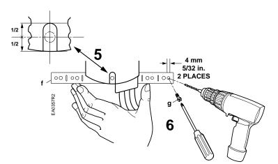
Anti-rotation tab should be approximately in the center of the actuator anti-rotation slot.
