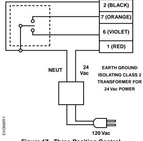
Figure 17. Three-Position Control.
