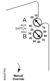
Figure 13. Dual Auxiliary Switch Dials.
