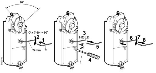
**Rotating** Turn the key in the direction of the arrow on the hand symbol. **Locking in place** Rotate the gear train lock pin. **Releasing when power is absent** Turn the key in the direction of the arrow.
