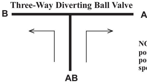
**NOTE:** View is from top of assembly, ports are marked. On 1/2" valves, port A is the limited Cv port, unless specified otherwise.
